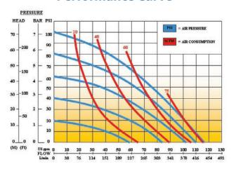
AIR PRESSURE: Tested at 100 psi / 690 kPa (not to exceed 125 psi / 861 kPa)
