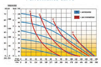
AIR PRESSURE: Tested at 100 psi / 690 kPa (not to exceed 125 psi / 861 kPa)
